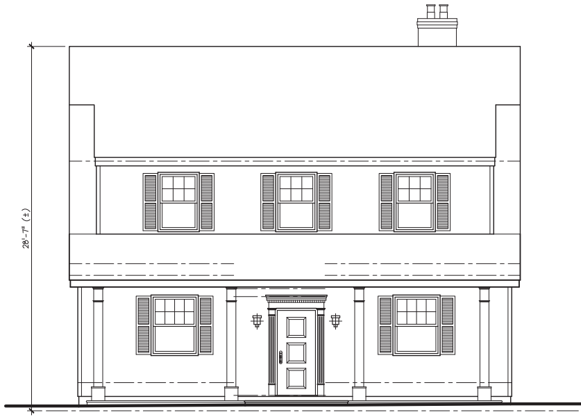
1 WEST (FERN STREET) ELEVATION EX-002 SCALE: 1/4" = 1'-0"
