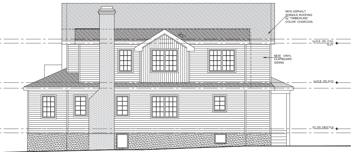
RIGHT ELEVATION (S-W) SCALE: 1/4"=1'-0"
