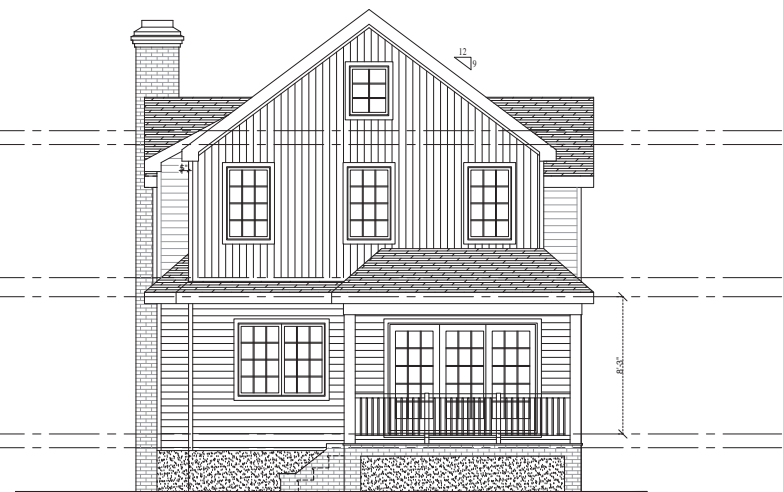
REAR ELEVATION (S-E) SCALE: 1/4"=1'-0"
