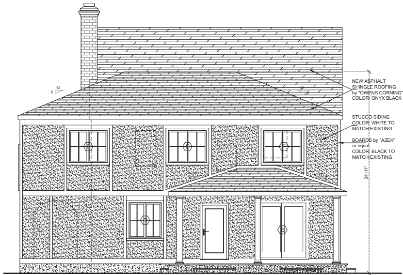
REAR SIDE (SW) ELEVATION APPROVED by ARB 4/26/23
