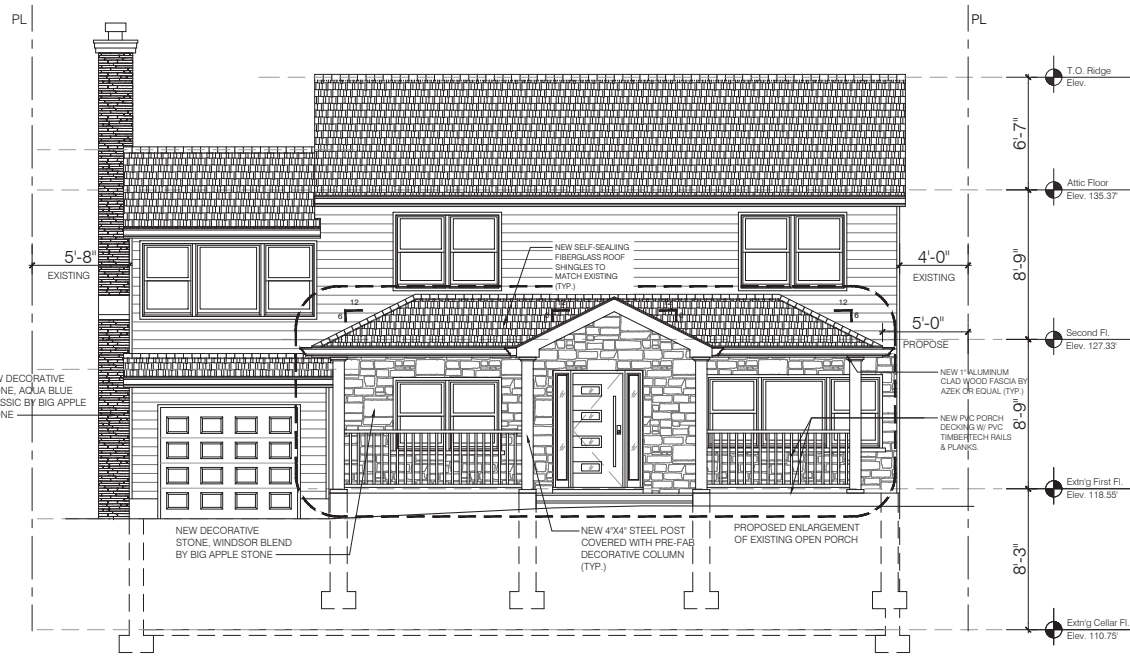
FRONT BUILDING ELEVATION PROPOSED SCALE: 1/4" = 1'-0"
