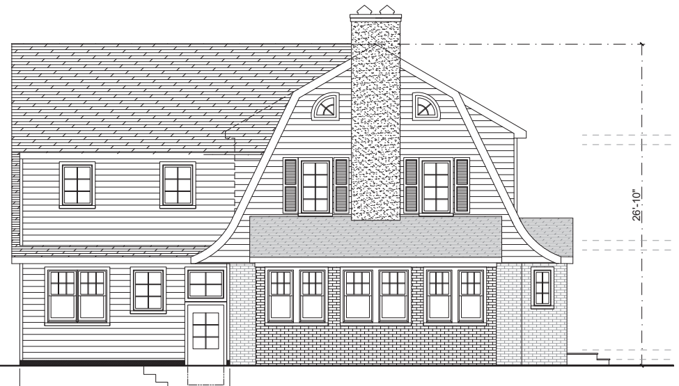
LEFT SIDE (E) - REMSEN LANE ELEVATION
